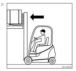
Lift the fork carriage until the load is resting entirely on the forks.
