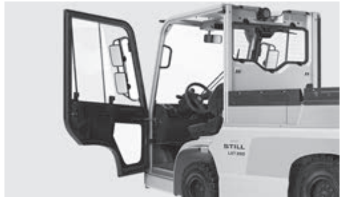
The robust operator's cabin is spacious and can be flexibly configured, e.g. with different doors or additional mirrors
