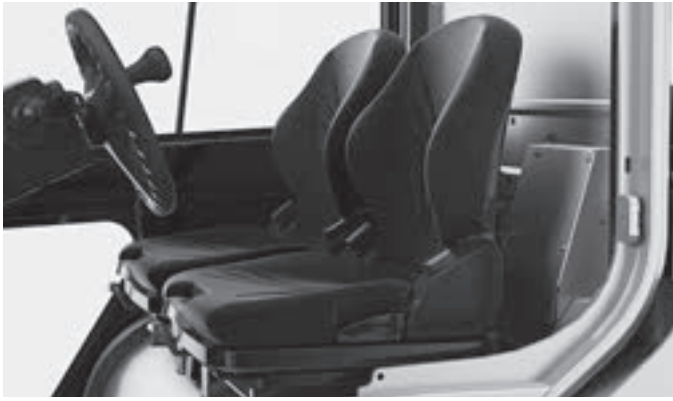
Working comfort in a class of its own with optional MSG 75 air sprung seat: Superior suspension on cushioned and sprung chassis
