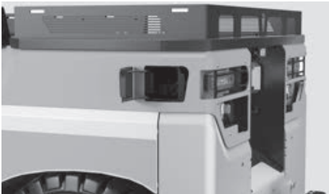
Safe and fast charging without opening the battery door thanks to the optional quick charging flap
