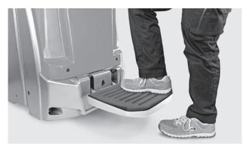
Back-friendly: air-sprung stand-on platform can be adjusted to individual driver's weight
