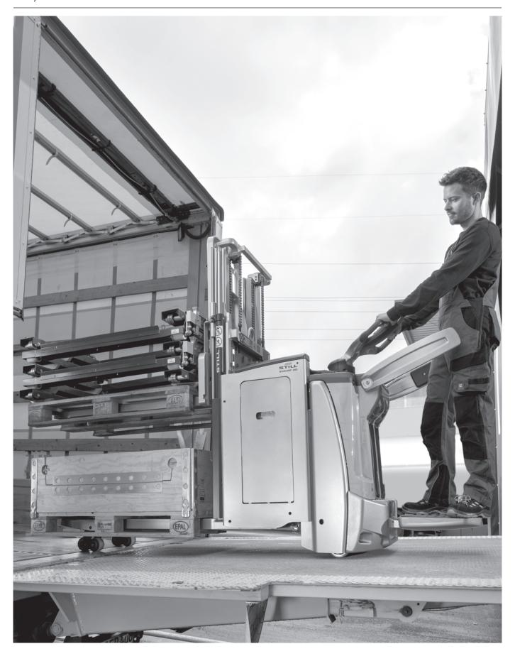
Speeds of up to 10 km/h and a maximum lifting capacity of up to 2,000 kg enable high handling rates
