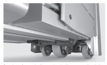
Convenient performance: handles power-intensive drives up ramps with optimal traction thanks to dampened support rollers  $\,$
