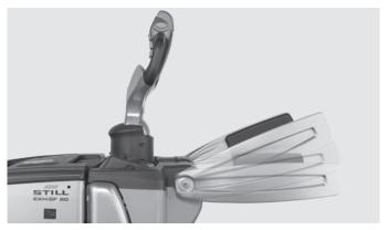
All-round safety: height-adjustable side guards provide optimal protection and stability
